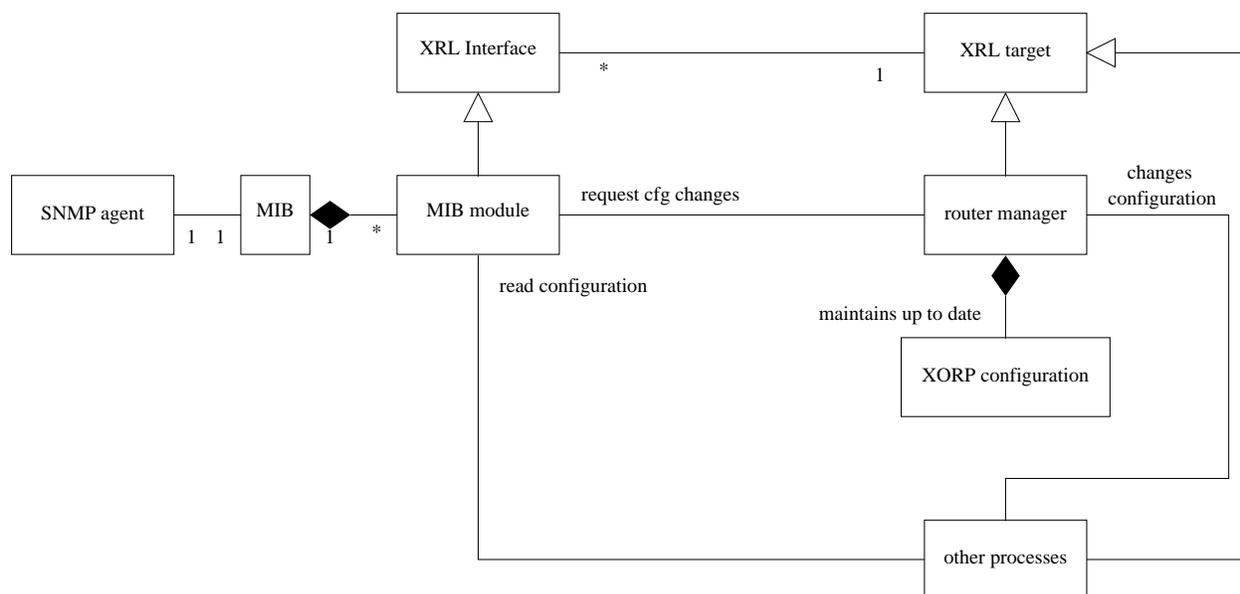
Figure 2: MIB module interactions with the router manager
