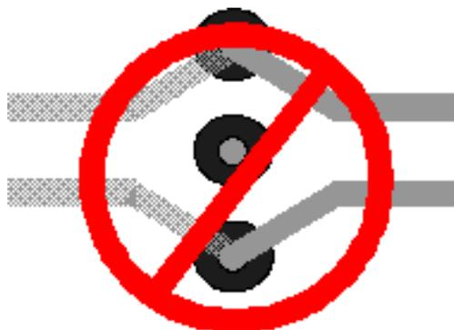
Figure 8-4. No Vias Between High-Speed Traces
