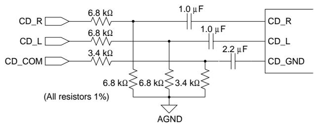
**Figure 19. Differential 2 V<sub>RMS</sub> CD Input**
