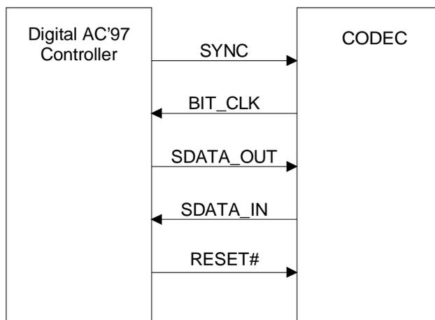
**Figure 7. AC-link Connections**
