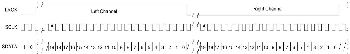
**Figure 13. Serial Data Format 2 (Right Justified, 20-bit data)**
