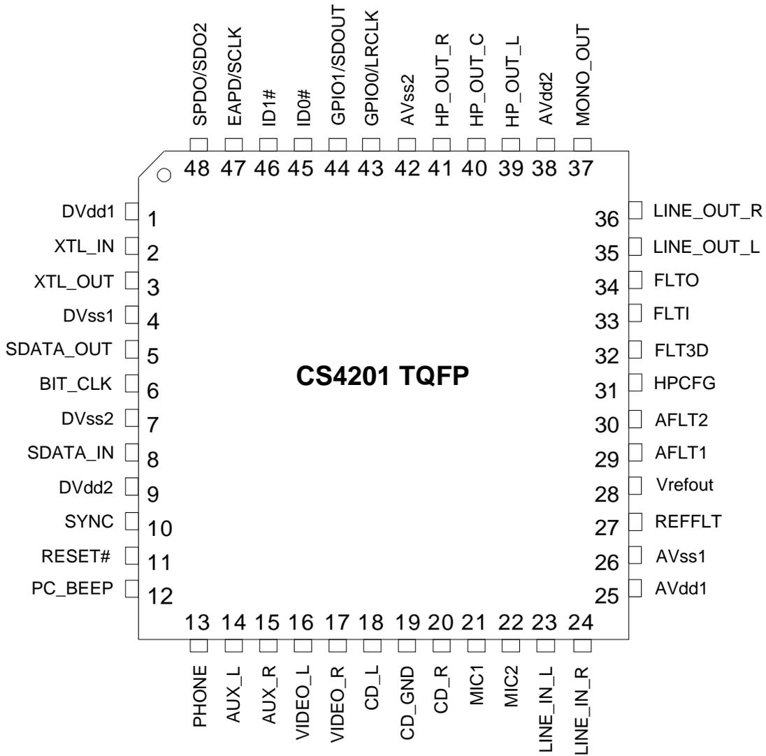
**Figure 28. Pin Locations for the CS4201**
