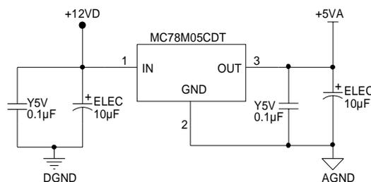
**Figure 26. +5V Analog Voltage Regulator**
