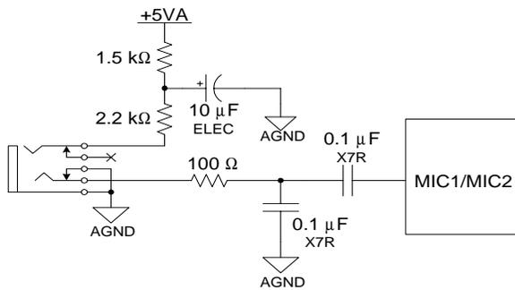
**Figure 21. Microphone Input**
