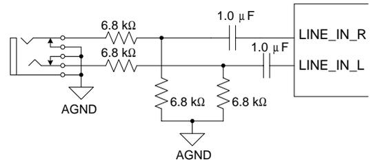
**Figure 18. Line Input (Replicate for Video and AUX)**
