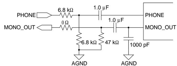
**Figure 23. Modem Connection**
