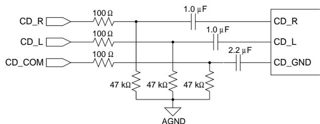
**Figure 20. Differential 1 V<sub>RMS</sub> CD Input**
