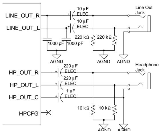
**Figure 24. Line Out and Headphone Out Setup**
