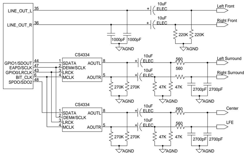
**Figure 10. Serial Data Port: Six Channel Circuit**
