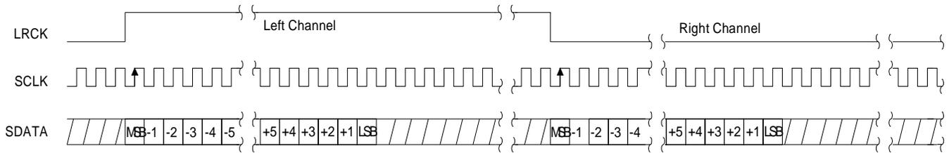
**Figure 12. Serial Data Format 1 (Left Justified)**
