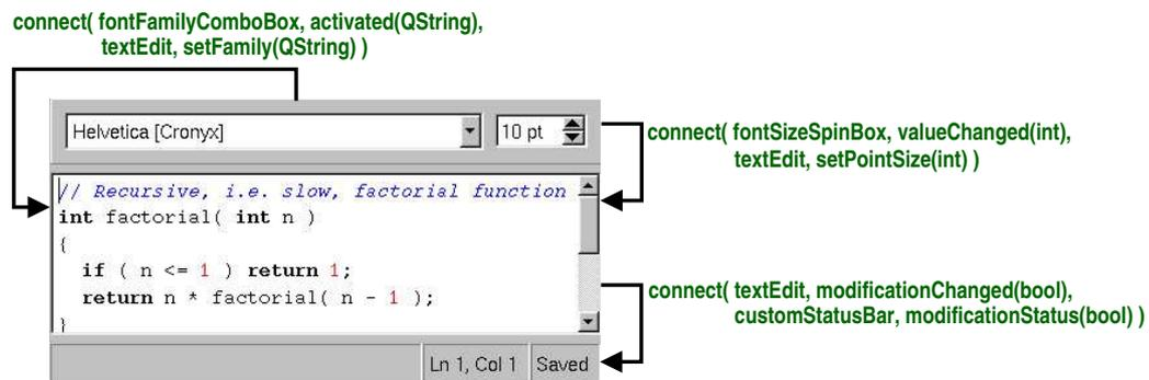
Figure 5. An example of signals and slots connections
